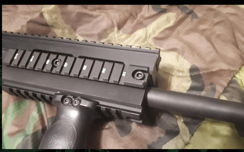
The forend has railed sections to allow the end user to add foregrips, flare launchers, flashlights, lasers and sling swivels all based on the individual end-user requirements. Specter Arms has an assortment of products to help get your S3 Phantom read for whatever mission you see fit.
