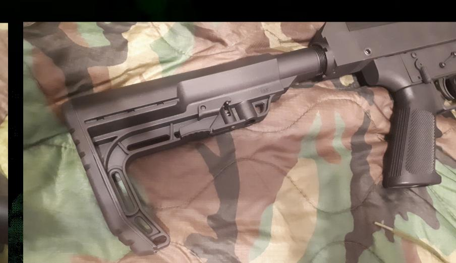
The S3 Phantom was designed to build a more balanced pistol caliber rifle. A common problem with this class of firearm is the long barrel combined with all the reciprocating mass in the center and a light (typically folding) stock. This makes a gun front-heavy and un-maneuverable.
