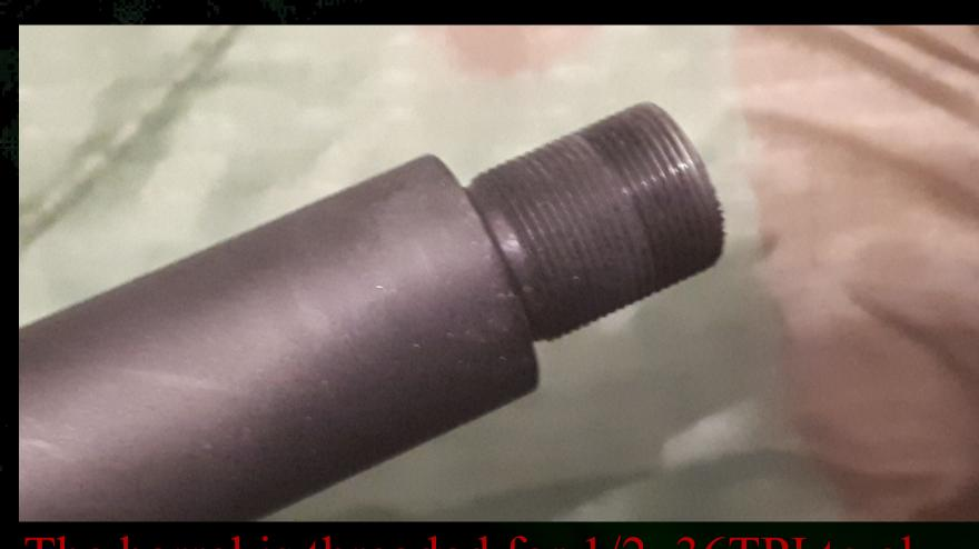
The barrel is threaded for 1/2x36TPI to allow for a variety of muzzle devices.
